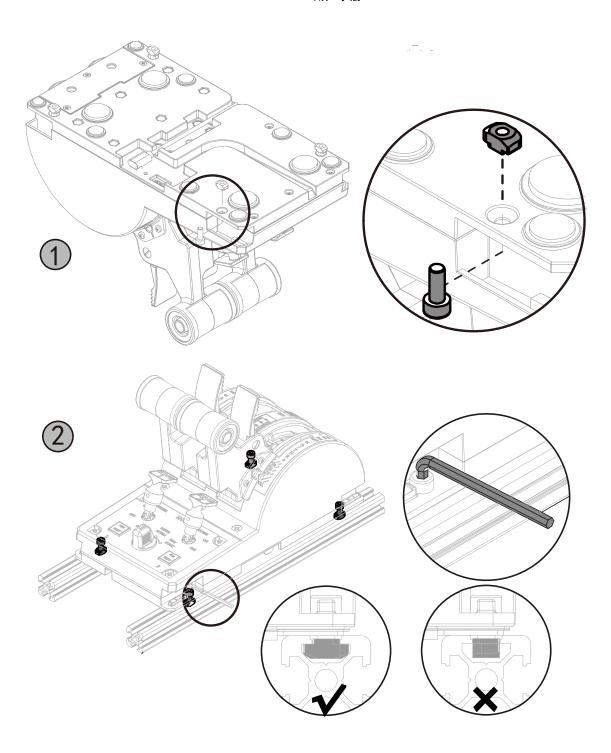
Flip the product. Insert the M4\*12 screw diagonally through the hole and screw in the M4 nut (2-3 turns will do);
