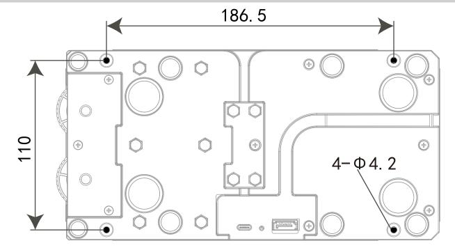
• The spacing of the assembling holes  $4-\emptyset$  4.2 is 186.5mm\*110mm.
