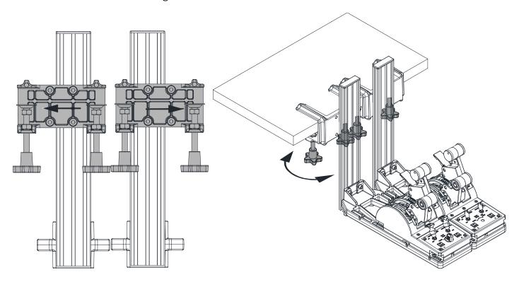
• After connecting the two products to the mounts respectively, remove them from the clamps and install them by translating 20mm, which is the distance of one slot (the left mount clamp is translated to the left, and the right mount clamp is translated to the right);
