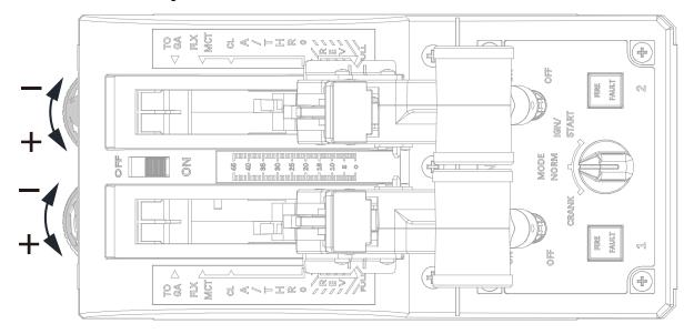
Counterclockwise rotation of the roller increases throttle shaft resistance, clockwise rotation reduces throttle shaft resistance.
