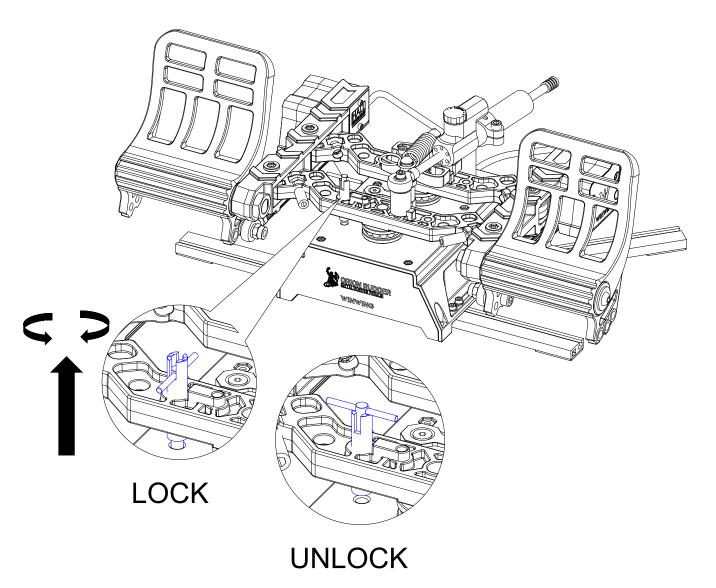
① Pull up the T-Handle pin as shown in the diagram and rotate it to the groove
