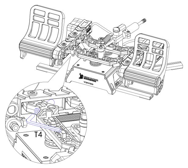
1) As shown in the diagram, the Glue Jackscrew can be adjusted on one side. Turning the Allen wrench counterclockwise unscrews it, while turning it clockwise screws it in
