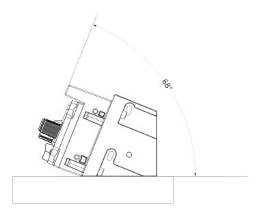
Insert USB data cable, set cable into the slot, and mount it to bracket using the R Shape
