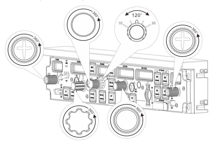
1.2.2 5 knobs, with rotation angle of 360° (no detent). NOTE: Only rotate is allowed, do not push/pull. Push/pull with excessive force may result in product damage.
