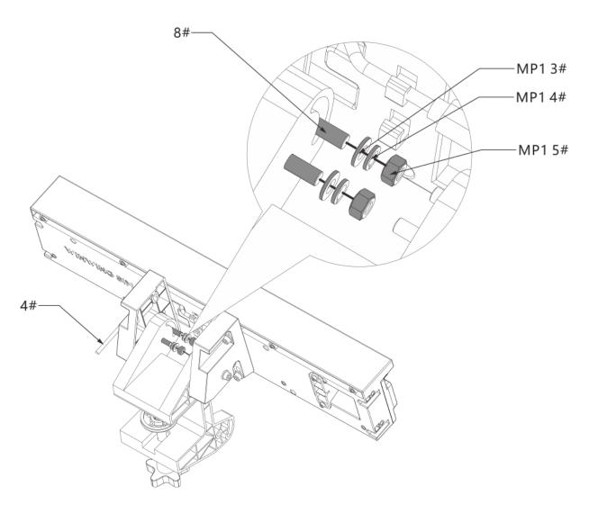
• Tighten the screws until there is no wobbling; over-tightening may cause damage;
