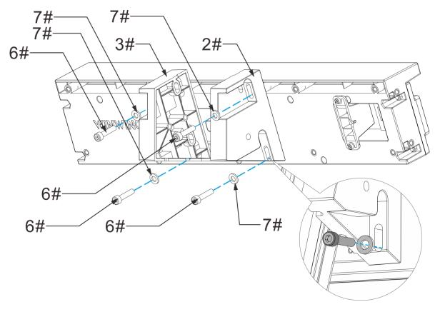
Tighten the screws, making sure the bottom of long form holes on 2# bracket and 3#
