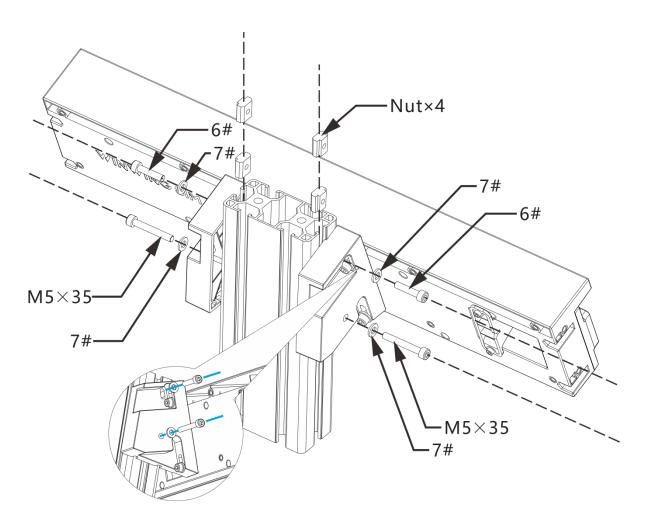
Put in profile nuts, adjust product position, then tighten the screws.
