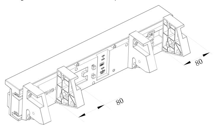
• Diagram above is between-bracket dimensions after brackets installed
