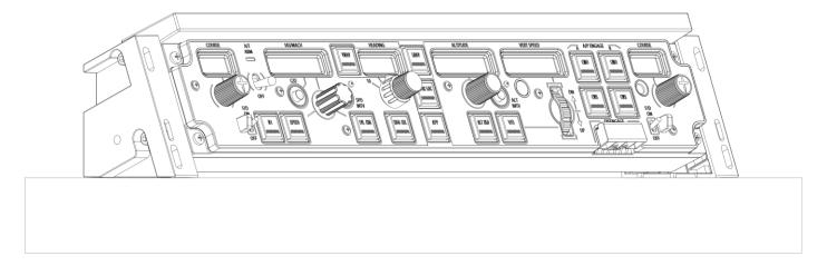
Insert USB data cable, set cable into the slot, and mount it to bracket using the R Shape
