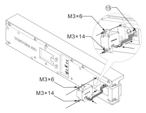
Insert one side of 7pin signal cable to Magnetic Switch, another side to ⑤ Reserved Magnetic Switch Port.
