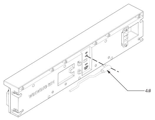
Insert USB data cable, set cable into the slot, and mount it to bracket using the R Shape
