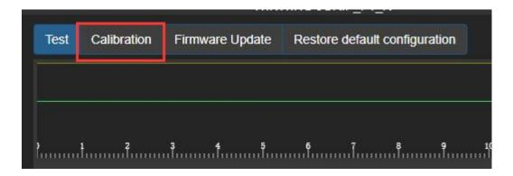
20n the calibration page, click the two buttons below to start calibration, then move the joystick through its full range.
