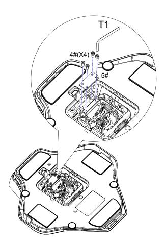
\*As shown in the figure, use a T1 (2.0mm) hex wrench: Secure the 1 lock plate with 4 M2.6\*8 self-tapping screws to lock the X-axis, and remove the lock plate to achieve X-axis rotation of  $\pm 15^{\circ}$ .
