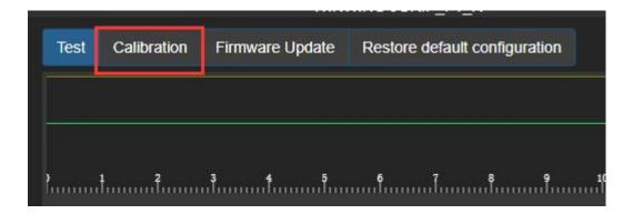
20n the calibration page, click the two buttons below to start calibration, then move the mini joystick through its full range.
