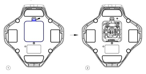
\*Flip the product to the bottom side, unfasten the clips and remove the bottom cover.
