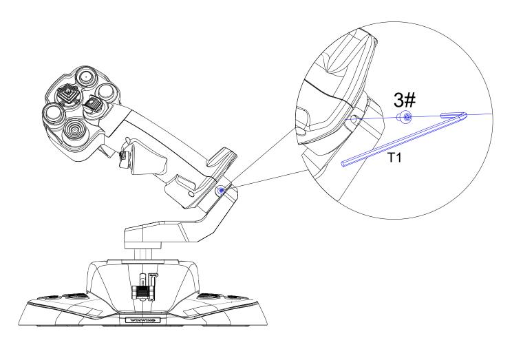
\*Z-axis is adjustable: With a T1 (2.0mm) hex wrench, tighten the screw to lock the Z-axis, and remove the screw to achieve Z-axis rotation of  $\pm 20^{\circ}$ .
