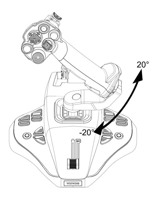
\*Z Axis Rotation Angle:  $\pm 20^{\circ}$  , Rotation Torque:  $^{\sim}4kgf \cdot cm$
