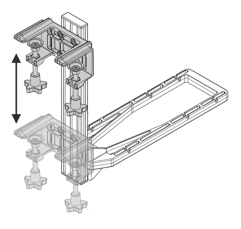
1.Both the MTX bracket and the clamping bracket 2 can be adjusted up and down within the slide groove of the profile, with an adjustment travel of ≥200mm. Excessively high or low positions may impact usability. Please adjust according to your actual needs.
