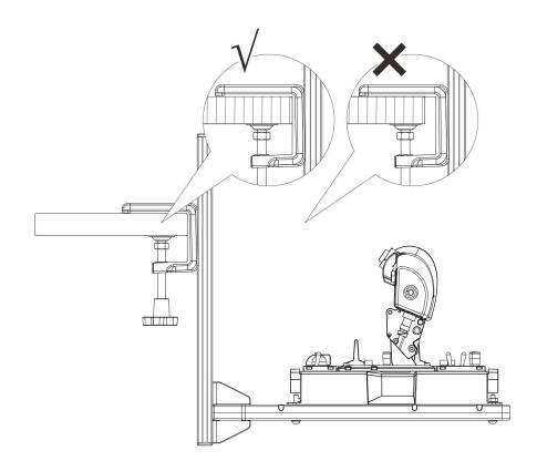
Clamp the mount on the table and alternate tightening the handle bolts left and right with a torque of 2.5N·m.
