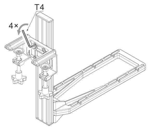
Loosen the screws by half to one turn.
