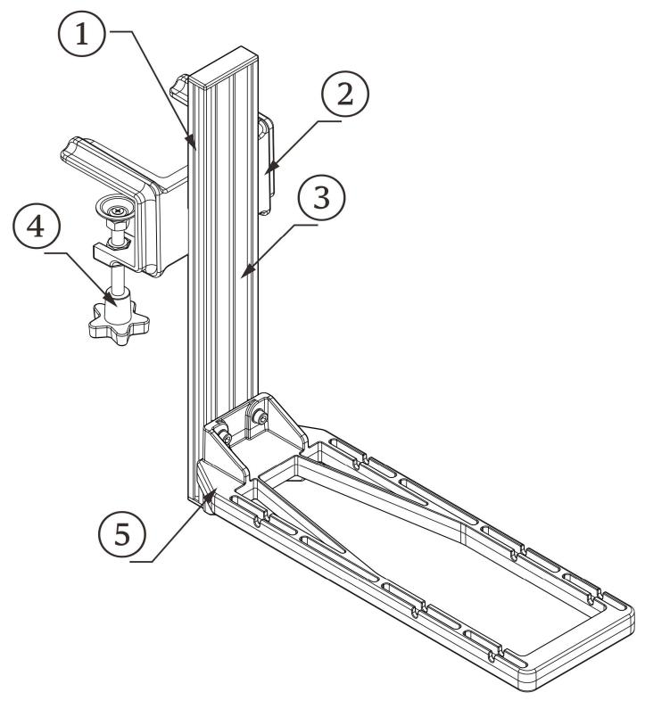
① Bracket pad mounting slot ② Clamping bracket ③ Profile assembly ④ Handle bolt ⑤ MTX bracket
