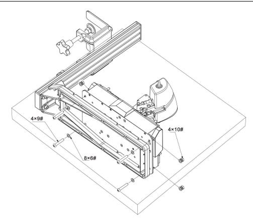
Place the Orion 2 NavyAce Throttle Combo on the MTX bracket, adjust the front and back positions, and then tighten the screws.
