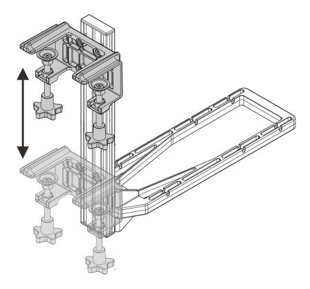
After adjusting the bracket up and down to the proper position, tighten the screws.
