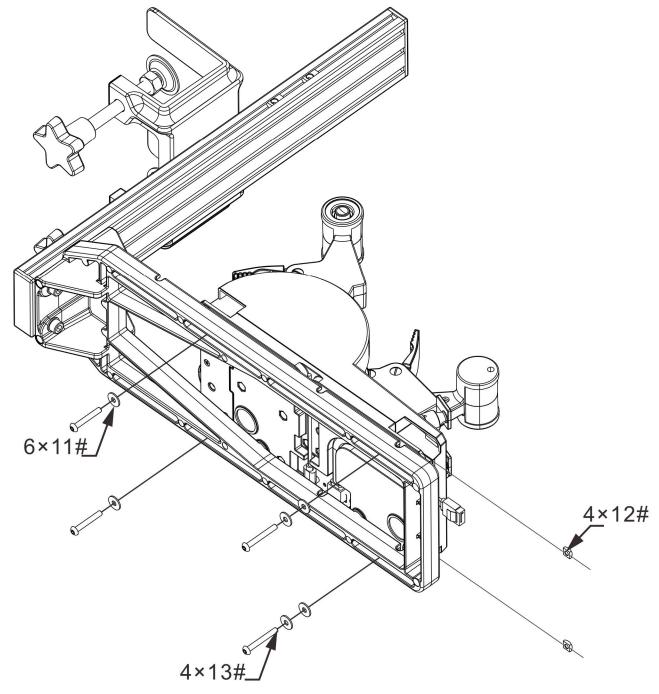
• Place the Ursa Minor Airline Throttle on the MTX bracket, adjust the front and back positions, screw in but do not tighten yet.
