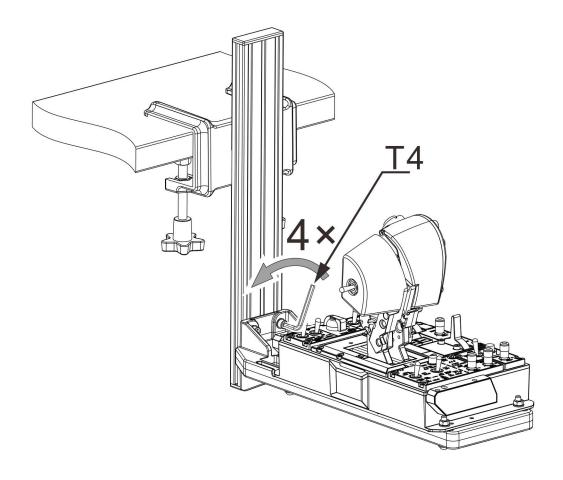
Loosen the four screws that connect the profile to the MTX bracket, adjust the MTX bracket up and down to a suitable height and tighten the screws.
