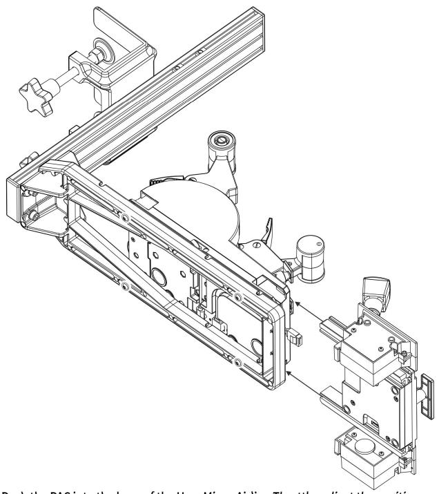
Push the PAC into the base of the Ursa Minor Airline Throttle, adjust the position and then tighten the screws.
