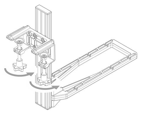
Rotate the handle bolt until the opening size of the clamp is close to the thickness of the desktop.
