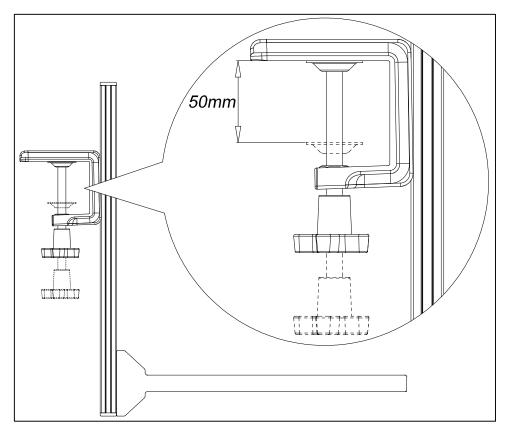
The thickness of the desktop should be  $\leq$  50mm, and the desktop compressive strength should be  $\geq$  1.8 MPa. (1. Depending on the material, clamping may cause indentations, scratches, or deformation. Perform a trial fit first, gradually increasing clamping force to assess acceptable limits. 2. Desktops must resist flexing, as deformation may lead to
