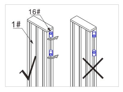
Insert the profile nut into the profile slot (note the direction of the profile nut).
