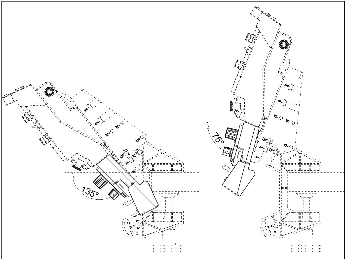
After connected with UFC1, it can be mounted on the clamp holders(need per chance), with an initial adjustable angle, adjustable range: 60 degrees.
