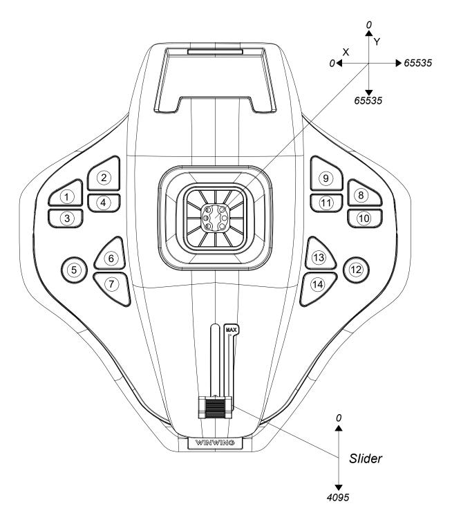
14 Button Switches: Press force of 250gf, Press travel of 0.25mm; Note: Please press the center area of the keycap. Pressing too close to the edge may cause the keycap to get stuck.
