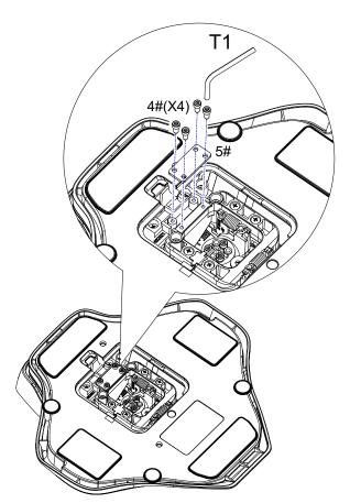
\*As shown in the figure, use a T1 (2.0mm) hex wrench: Secure the 1 lock plate with 4 M2.6\*8 self-tapping screws to lock the X-axis, and remove the lock plate to achieve X-axis rotation of  $\pm 15^{\circ}$ .
