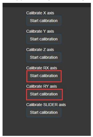
③After moving, let the mini joystick naturally return to the center, then click the two buttons below.
