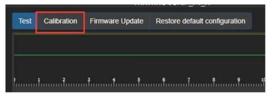
20n the calibration page, click the two buttons below to start calibration, then move the mini joystick through its full range.
