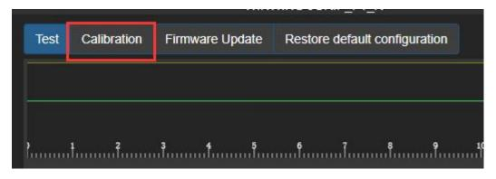
20n the calibration page, click the two buttons below to start calibration, then rotate the Z-axis through its full range.
