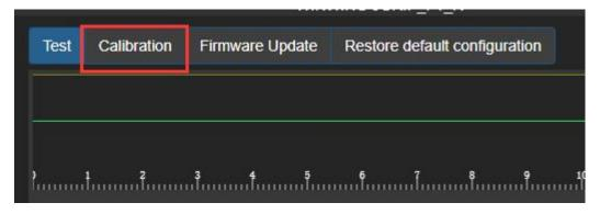
20n the calibration page, click the button below to start calibration, then move the slider axis through its full range.
