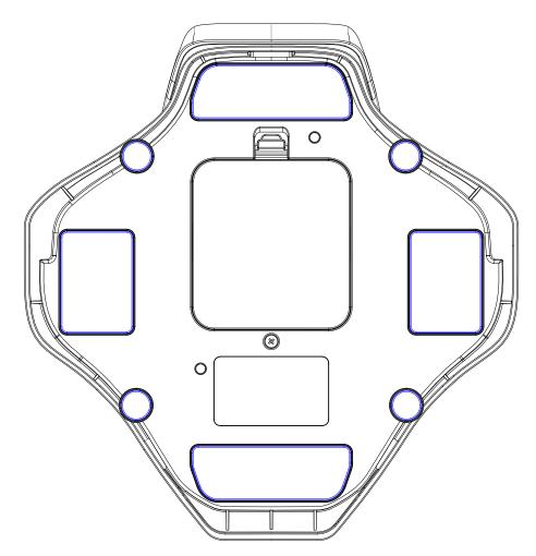
\* As shown, remove the protective film from the bottom silicone pad and place it directly on the desktop.
