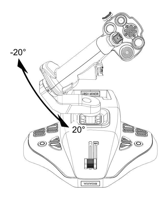
\*Z Axis Rotation Angle:  $\pm 20^{\circ}$  , Rotation Torque:  $^{\sim}4$ kgf  $^{\sim}$  cm.
