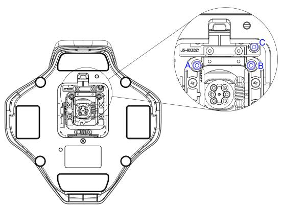
\* As shown, use T2 (2.5mm) hex wrench: Adjust screws A and B simultaneously to adjust Y-axis damping (clockwise to increase, counterclockwise to decrease). Adjust screw C to adjust X-axis damping (clockwise to increase, counterclockwise to decrease).
