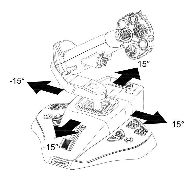
\*Axis Movement Angle:  $\pm 15^{\circ}$  , Operating Force:  $^{\sim}6N$ .
