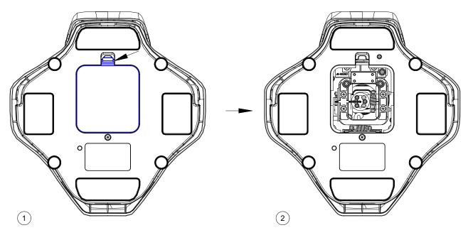
\* Flip the product to the bottom side, unfasten the clips and remove the bottom cover.
