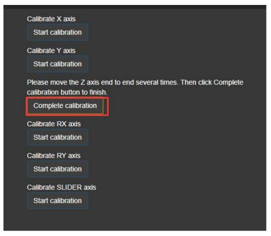
At this point, the Z-axis calibration is complete. Return to the test page and observe if the data is normal. If there are abnormalities, please re-execute the calibration steps.
