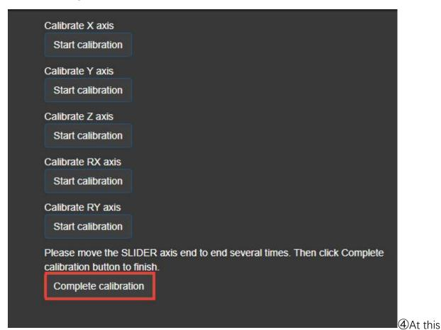
point, the slider axis calibration is complete. Return to the test page and observe if the data is normal. If there are abnormalities, please re-execute the calibration steps.
