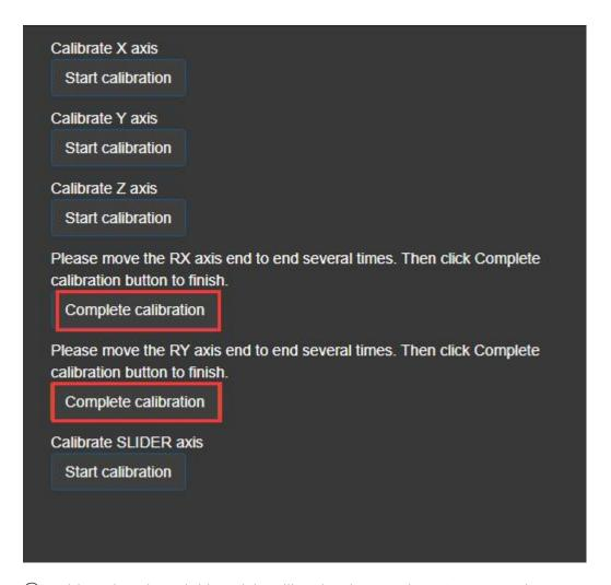
At this point, the mini joystick calibration is complete. Return to the test page and observe if the data is normal. If there are abnormalities, please re-execute the calibration steps.
