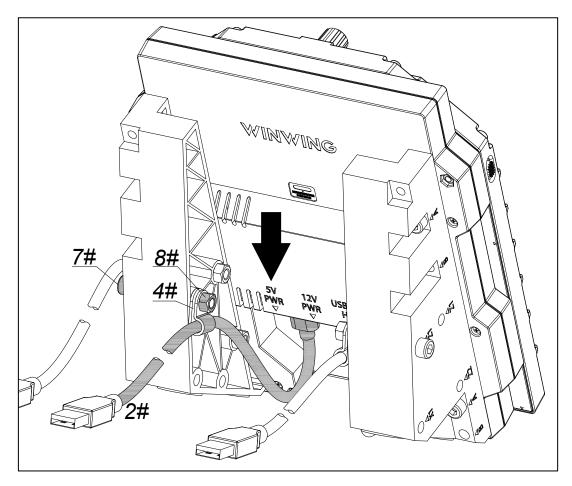
\*Please plug in the 2# cable (not provided) to the "5V PWR" socket (power supply only) to supply a 5Vpower when the device is failed to be identified.
