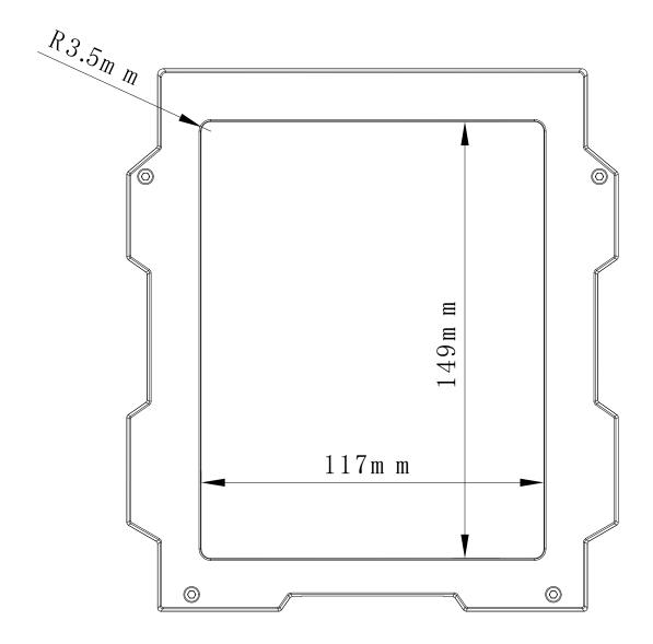
The product display area measures 117mm in width and 149mm in height; The screen resolution is 1024\*3 (RGB) \*768. Please note that this is the screen resolution, not the display area resolution.
