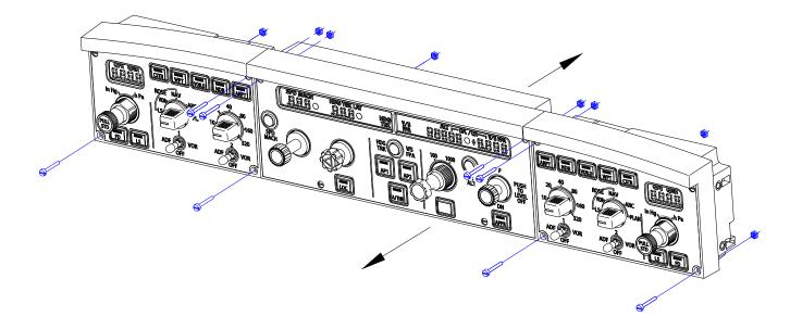
2. Install EFIS-32L on the cockpit frame; screw specifications are listed below:
