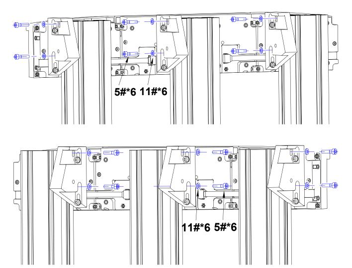
Above diagrams provide an overview of the 4080 profile mounting (profile rails and accessories need to be self-prepared).
