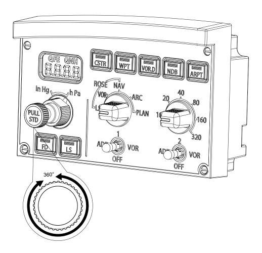
1) PULL STD Knob has a push-pull stroke of 2.5mm and can rotate 360° (without detents). Note: Only push, pull, and rotate; do not bend. Bending destructive force is 500gf. Maximum rotational torque is 150gf · cm, maximum push-pull force is 1200gf.
