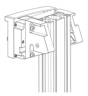
The diagram above shows the mounting method for the 4080 profile (profile rails and accessories need to be self-prepared).
