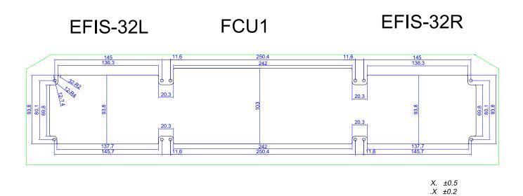
Cockpit Frame Drilling Diagram
