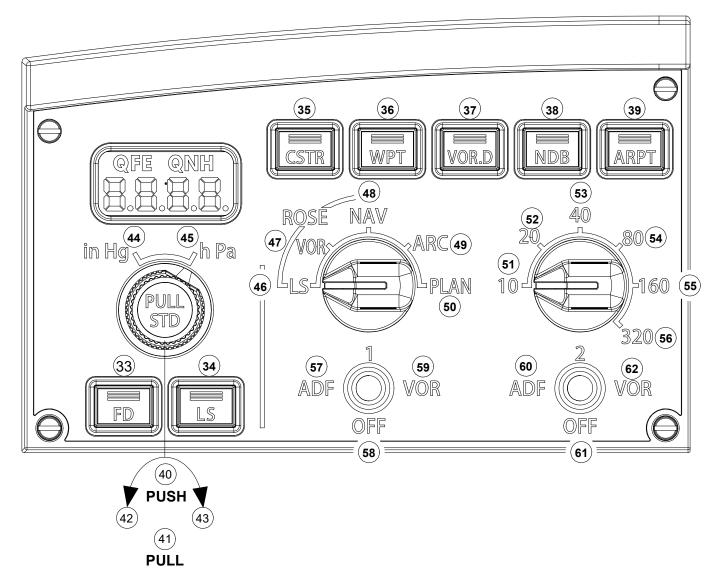
Keys 44, 45, and 42, 43 cannot be rotated simultaneously. When operating keys 44 or 45, rotation signals from keys 42 and 43 are automatically disabled.
