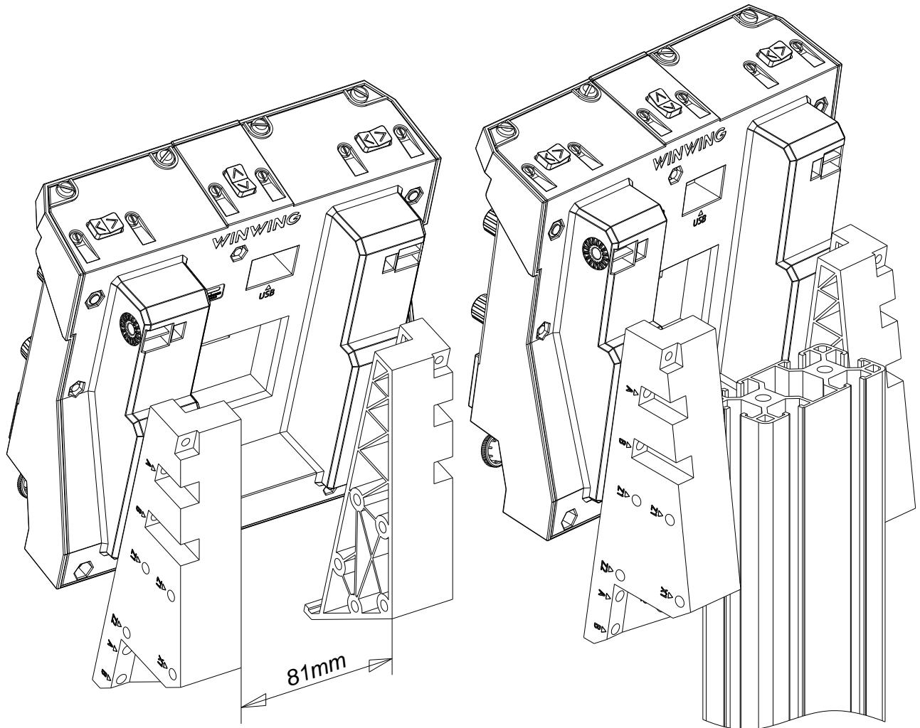
Can be mounted on 4080 aluminium profiles (Not provided). (Screw:M5\*40.M5 T-Nut for 40 Sereis Aluminum Profile)
