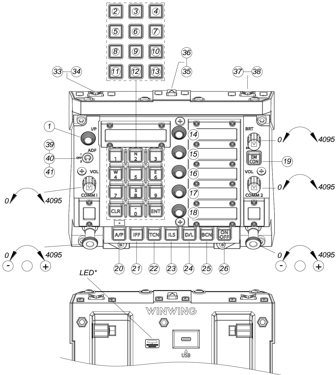
\* LED status: Steady slow flashing in green (1s interval) - BOOT mode.
