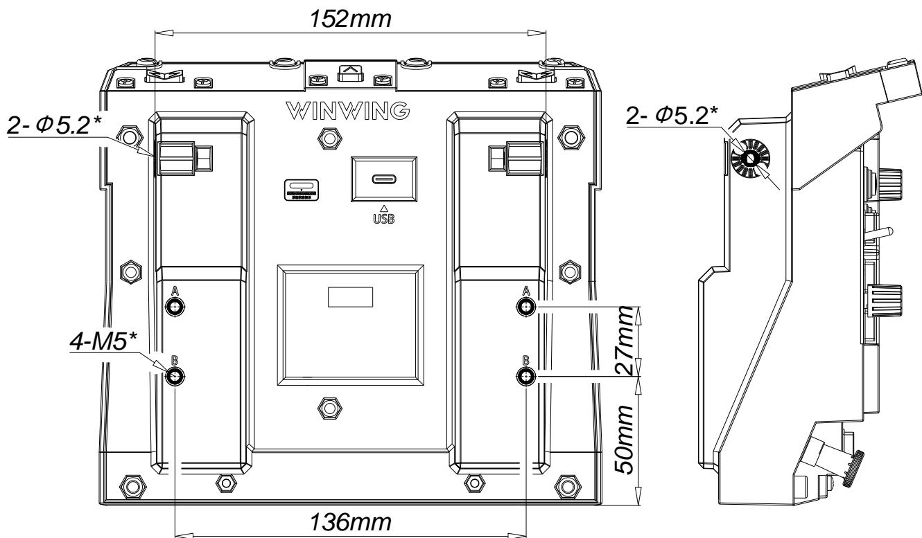
\*2-Φ5.2: Additional mounting holes ;4-M5 maximum depth: 5mm.
