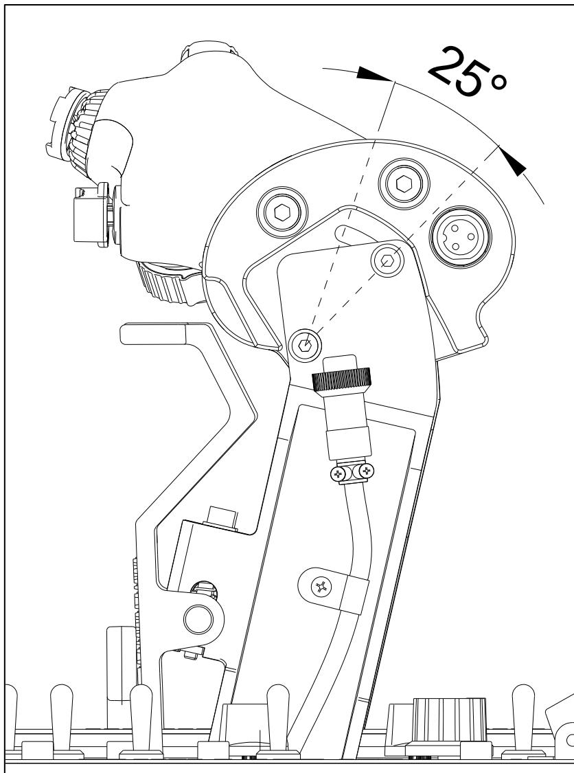
Adjustable angle for initial installation  $25^\circ$ .
