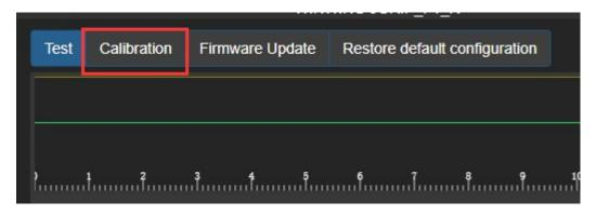
20n the calibration page, click the following two buttons to start calibration, and then move the joystick to the full travel;
