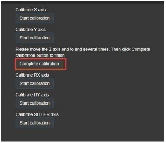
(4) After finishing step 3, the calibration of Z axis is completed. Go back to the te st page to check if the data is normal, if not, repeat the calibration steps.
