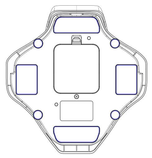
\* Remove the protective film from the bottom silicone pad as shown in the figure, and place it directly on the desk.
