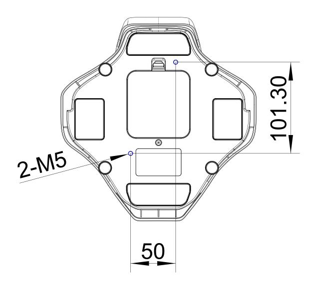
Note: The screw insertion depth must be greater than 6mm and less than 10mm. Screws must be self-supplied and are not included in the accessory kit.
