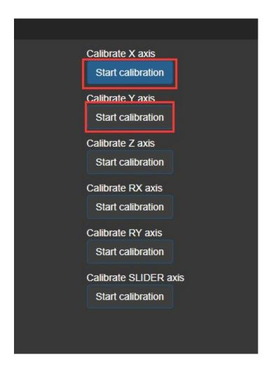
③After completing the movement, allow the joystick to naturally return to the center, and then click the two buttons shown in the following figure;
