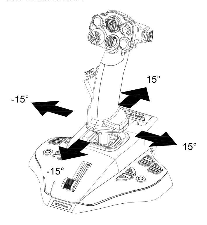
\*The X/Y axes have a movable angle of  $\pm 15^{\circ}$  , with an operating force of approximately 6 newtons.
