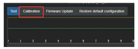
20n the calibration page, click the following two buttons to start calibration, and then move the mini joystick to the full travel;
