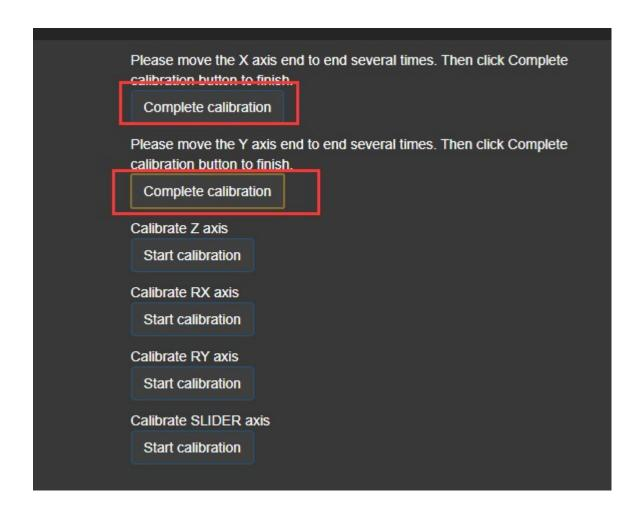
After finishing step 3, the calibration of joystick is completed. Go back to the test page to check if the data is normal, if not, repeat the calibration steps.
