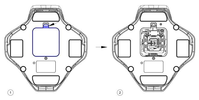
\* Turn the product upside down, release the latch, and remove the bottom cover.
