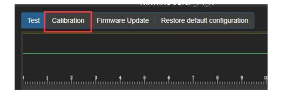
20n the calibration page, click the following button to start calibration, and then rotate Z axis to the full travel;
