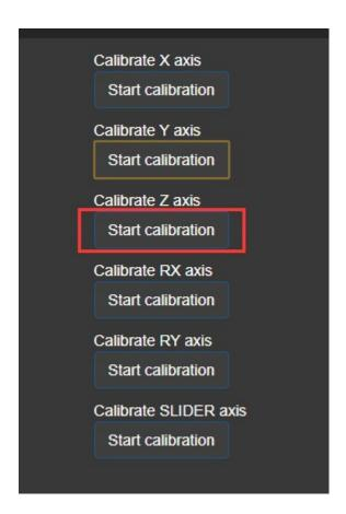
③After finishing step 2, make the Z axis return to the center naturally, and then click the following button;
