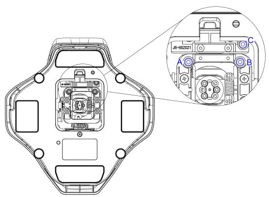
\* As shown in the figure, use the T2 (2.5mm) hex wrench: Adjust screws A and B simultaneously to control the Y-axis damping (increase damping clockwise, decrease counterclockwise); by adjusting screw C, you can control the X-axis damping (increase damping clockwise, decrease counterclockwise).
