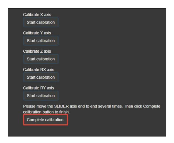
After finishing step 3, the calibration of Slider axis sliding block is completed. Go back to the test page to check if the data is normal, if not, repeat the calibration steps.
