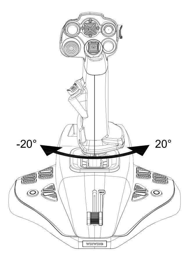
\*The Z axis has a rotational angle of  $\pm 20^{\circ}$  , with a rotational torque of approximately 4 kgf  $\cdot$  cm.
