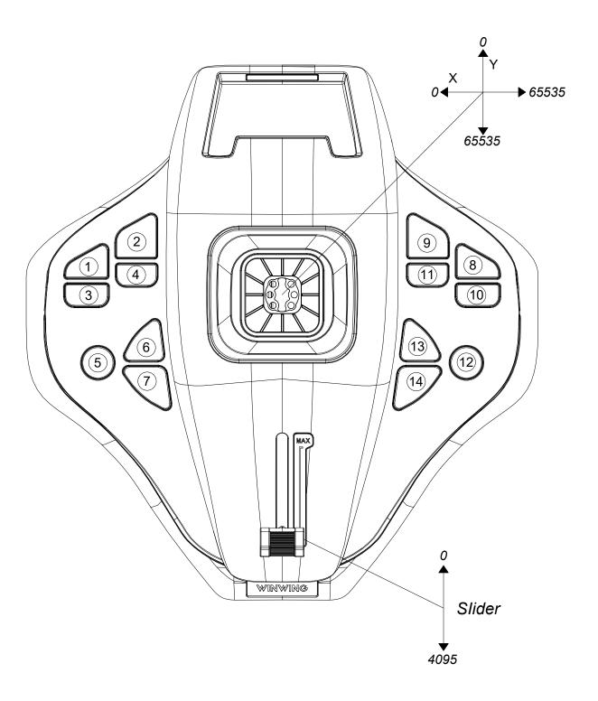
\*14 key switches with press force of 250gf and press travel of 0.25mm.
