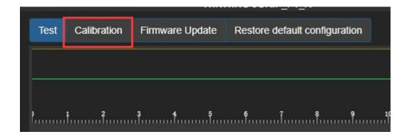
20n the calibration page, click the following button to start calibration, and then move the Slider axis sliding block to the full travel;
