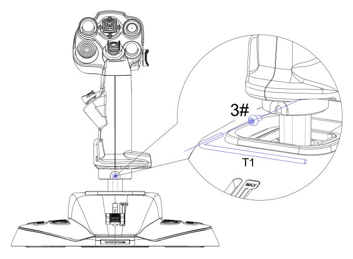
\*Adjustable Z-Axis: Use the T1 (2.0mm) hex wrench to tighten the screw, which will lock the Z-axis in place. Removing the screw allows for Z-axis rotation of  $\pm 20^{\circ}$ .
